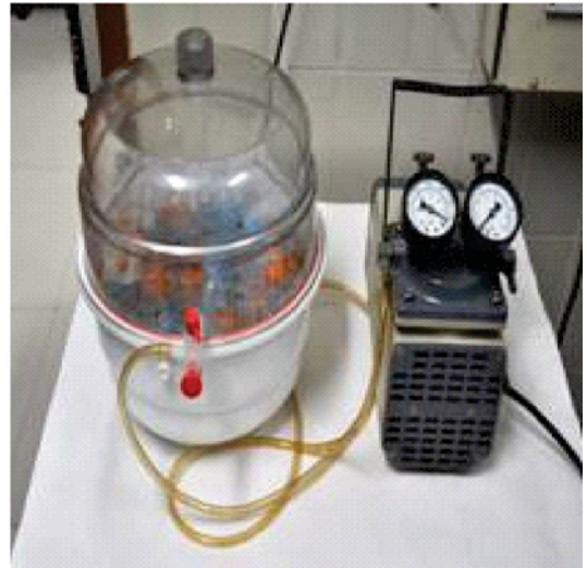
Fig B Vacuum desiccator for faster drying
