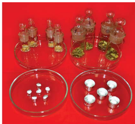
Fig. D Glass moisture bottles and Aluminium cups of different sizes
