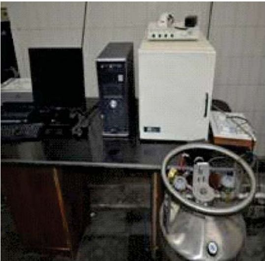
Fig. C Programmable rate freezing apparatus
